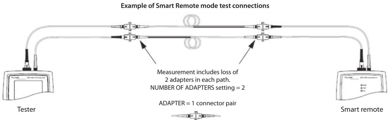
You must therefore enter the correct number of Adaptors in your link as well as the correct number of Splices, (within Patch Panels etc.) Underneath the Test Limit on the TEST SETUP Screen, there are 3 settings: Reference Method should always be 1 Jumper. The next is the Connector Type the last one covers the number of Connections/Splices, select this and it will bring up the next screen.
