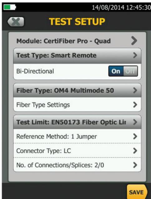
You will then have to change some of the other settings, ensure that Test type is SMART REMOTE and Bi-Directional is ON. Fibre Type is correct
